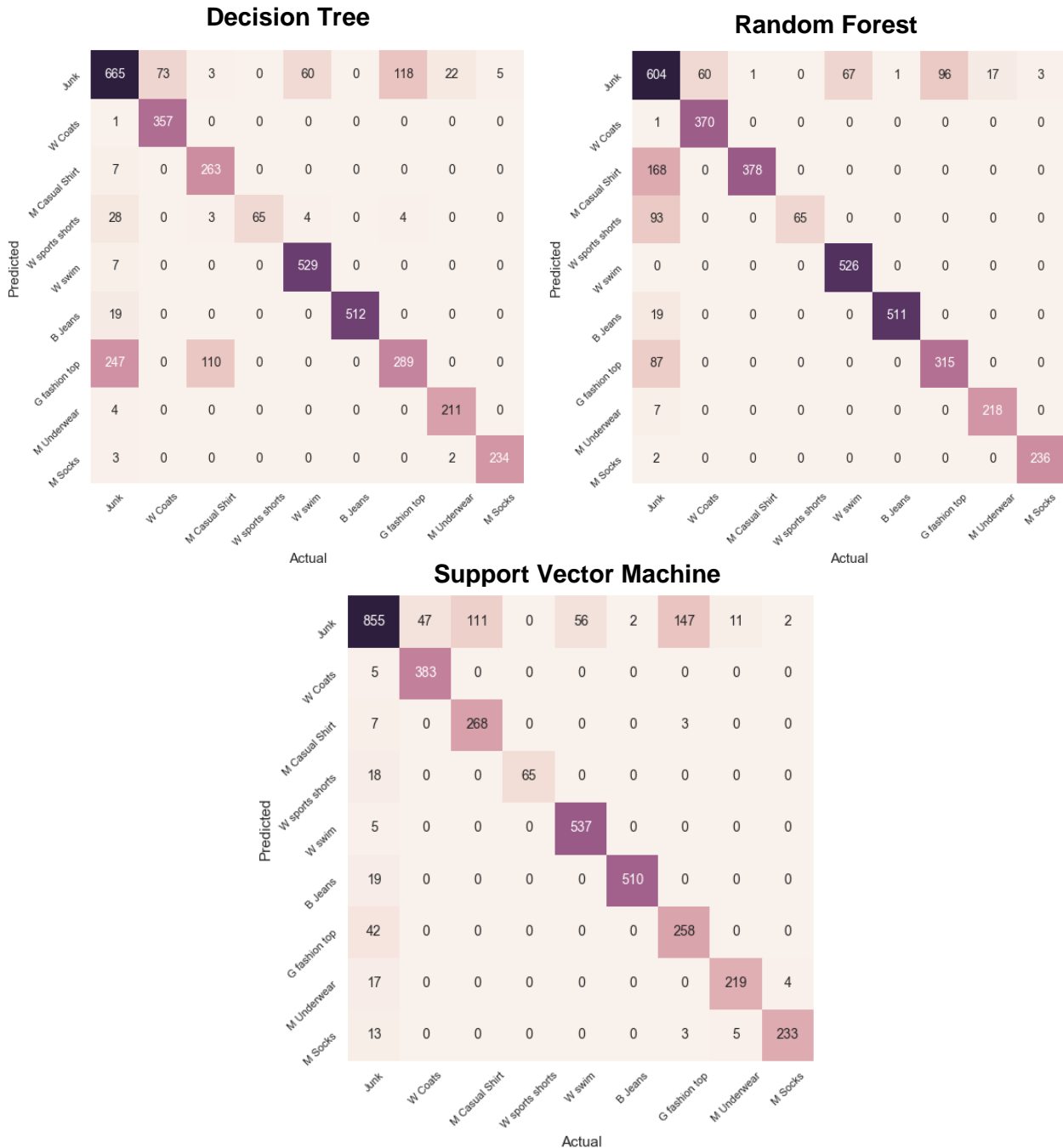
Figure 7: Confusion matrices for the three classification methods with TF-IDF vectors. Top left panel is the decision tree, top right random forest and bottom is the non-linear SVM. These are the confusion matrices for the test dataset.
